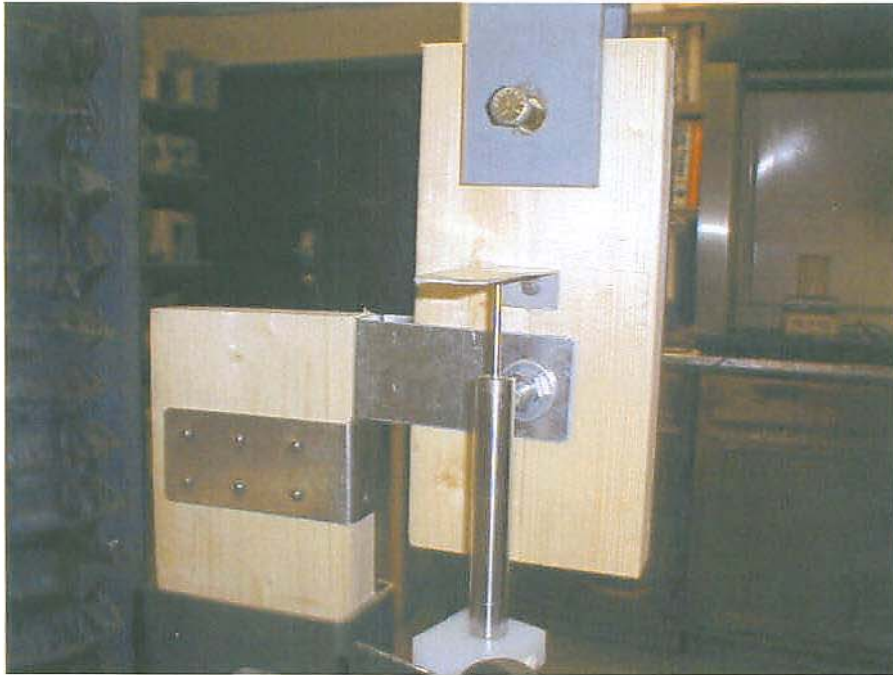
PHOTO 1: Test A, Lateral Test Specimen/Test Setup
