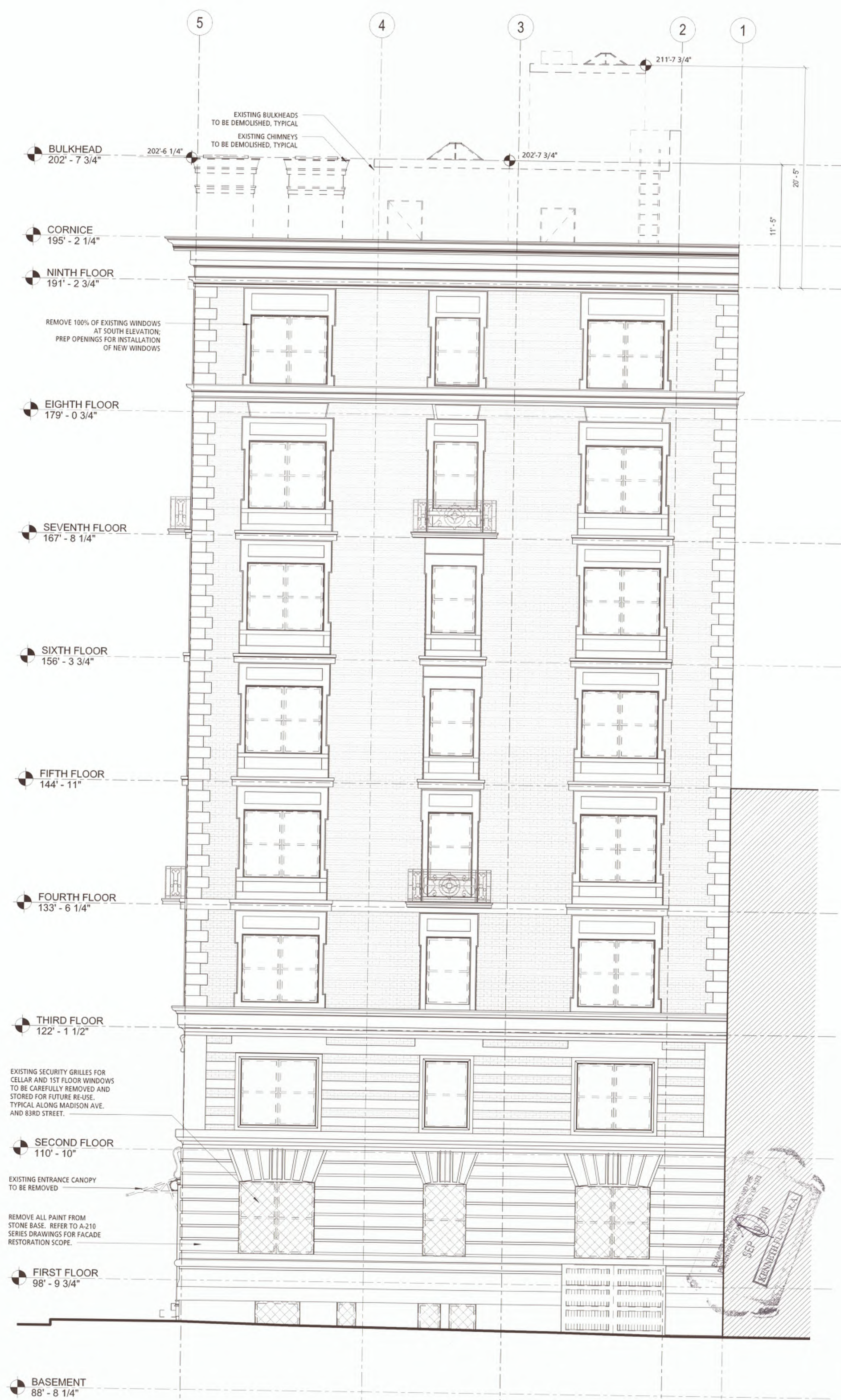
1 South Exterior Demolition Elevation 3/16" = 1'-0"
