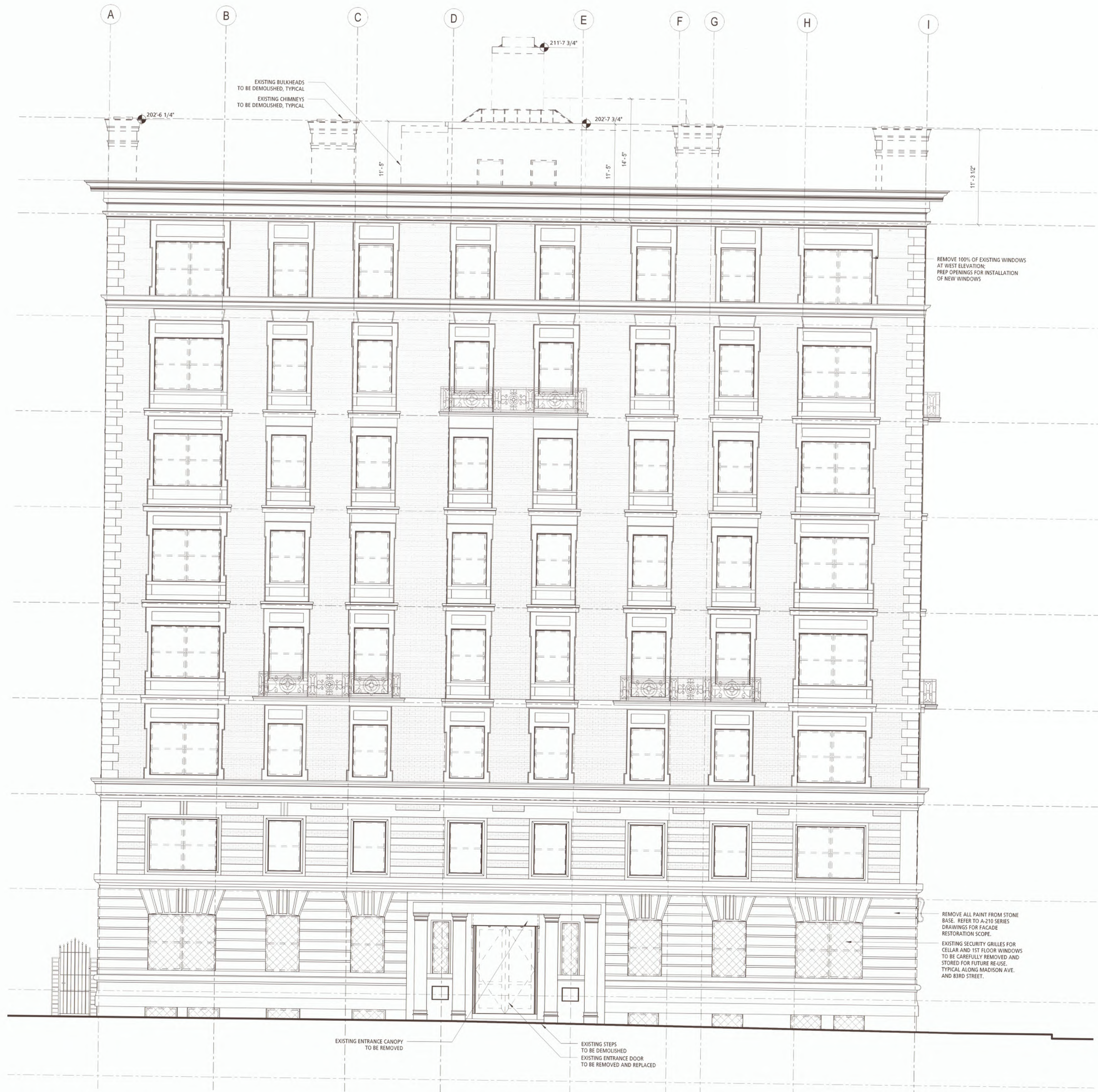
2 West Exterior Demolition Elevation 3/16" = 1'-0"
