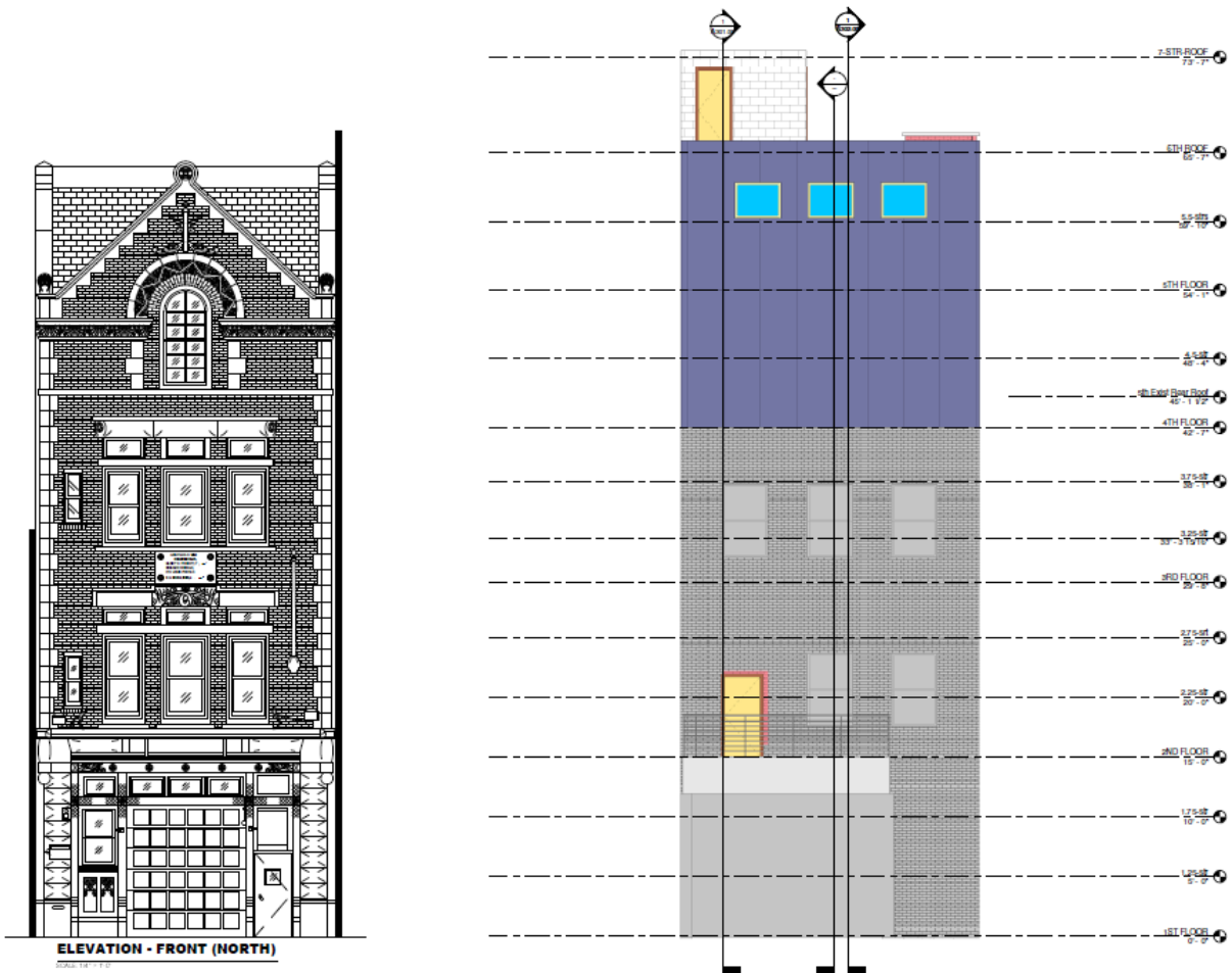
Figure 3-2 Proposed Structure Front and Rear Elevations
